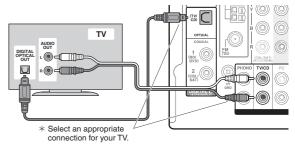
Another TV can be connected to the HDMI OUT SUB jack. In this case, change the setting accordingly. You can set up by viewing the guidance displayed on the TV screen. Select the item with the cursor buttons of the remote controller and press Enter to confirm your selection. Press RCV and then
